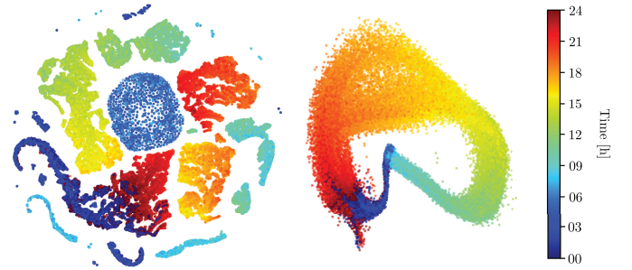
Fig. 3. Latent space visualization of \mathcal{X}_{\text{train}}^{\text{normal}} in 2D via t-SNE (left) and PCA (right). (on-line mode, training executed using overlapping sequences with T = 32 timesteps).
